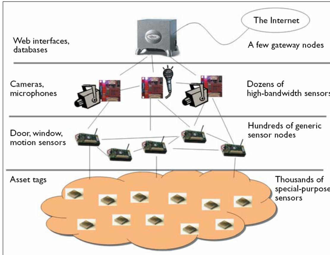
**Hierarchical deployment of a wireless sensor network. Each platform class handles different types of sensing.**
